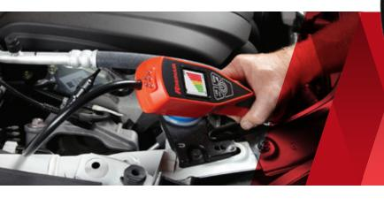
Leaking refrigerant, especially 1234yf, can be an expensive problem. Using a 5% hydrogen/ 95% nitrogen tracer gas mix can help find leaks faster for repair and recharge of the A/C system, without losing
