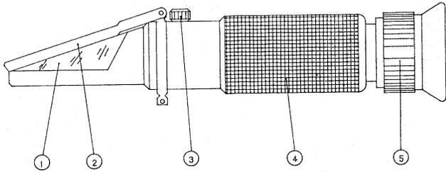
1. Aim the front end (prism [1] and cover plate [2] end) of the refractometer toward a bright light; then adjust the focusing ring of the diopter (5) until the reticle (scale within the mirror tube) can be seen clearly.
