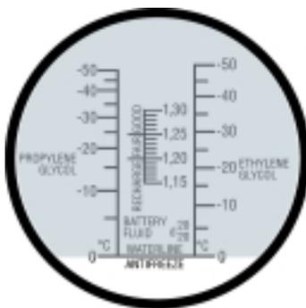
The Hand Refractometer should now have a null point, and you are ready to begin measuring.
