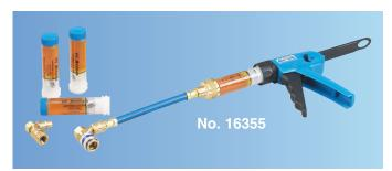
Simple to use: Twist a cartridge onto the injector gun, hook up to the service port, and pull the trigger to inject the dye into the A/C system. Put your old lamp to use to spot the leak and you're done.
